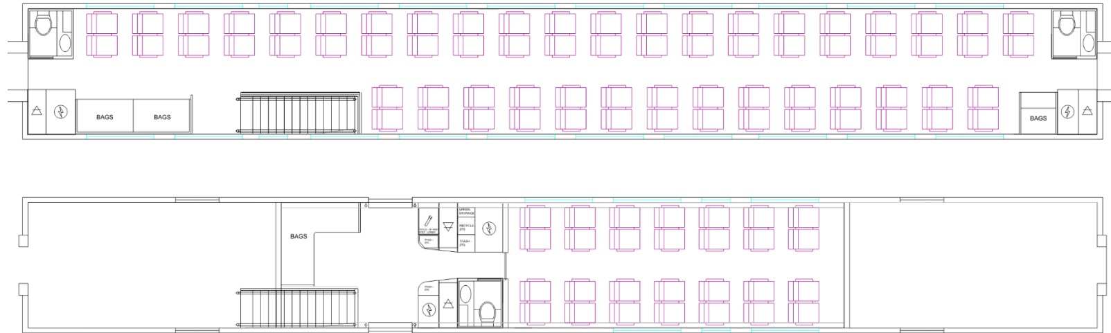
Figure 1-5: Conceptual Car Type Arrangement - End Coach
