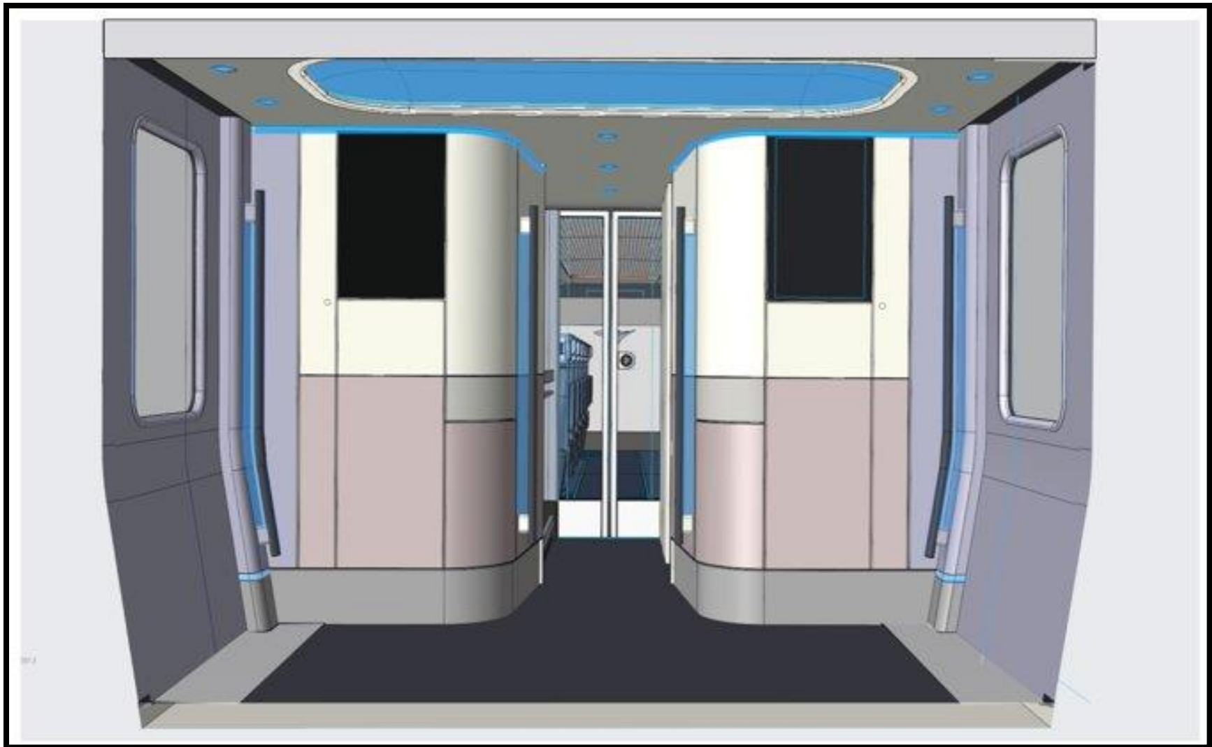
Figure 11-54: Entrance Area Light Locations
