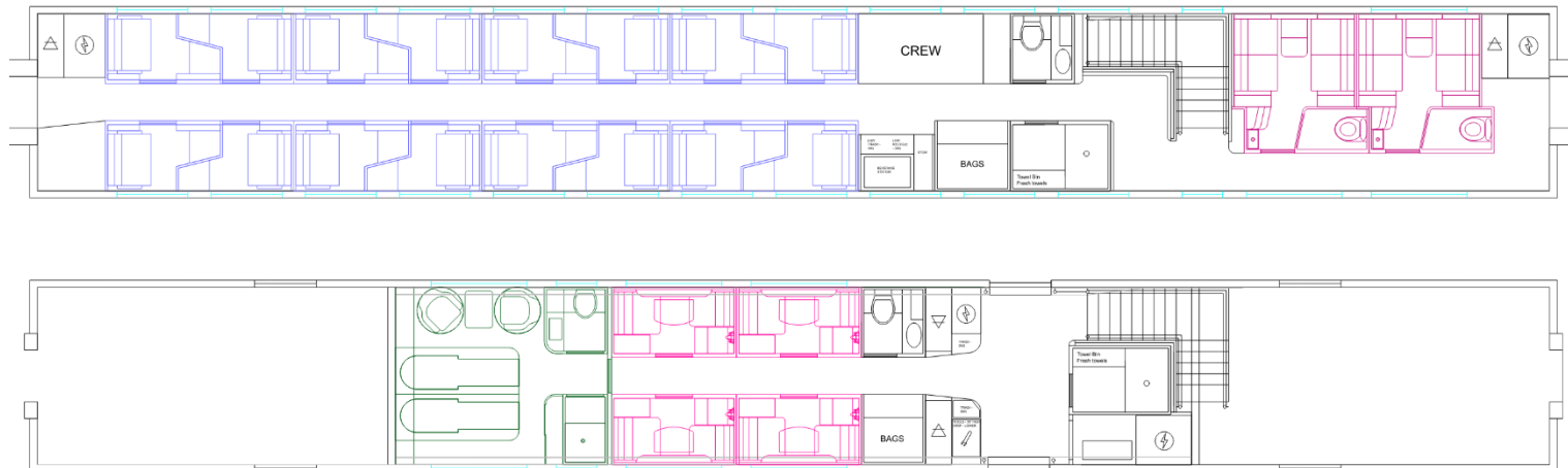
Figure 1-12: Conceptual Car Type Arrangement - Standard Sleeper
