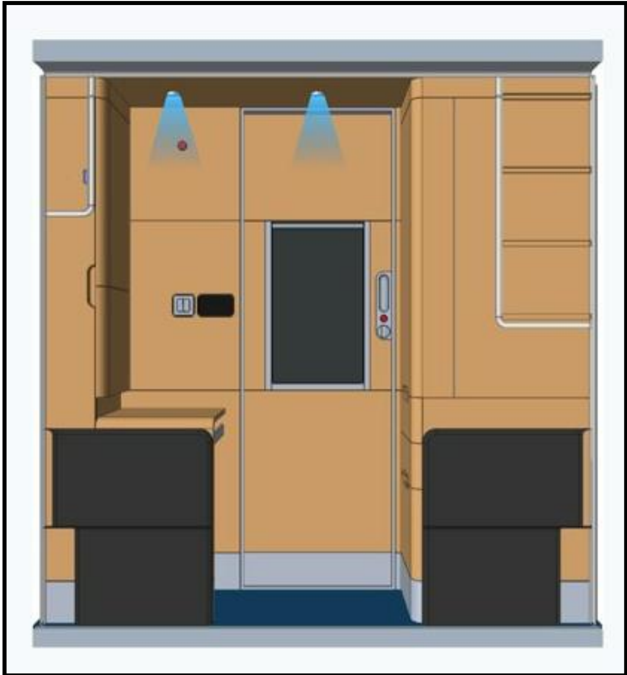
Figure 11-129: Crew Sleeper Spot Light Locations
