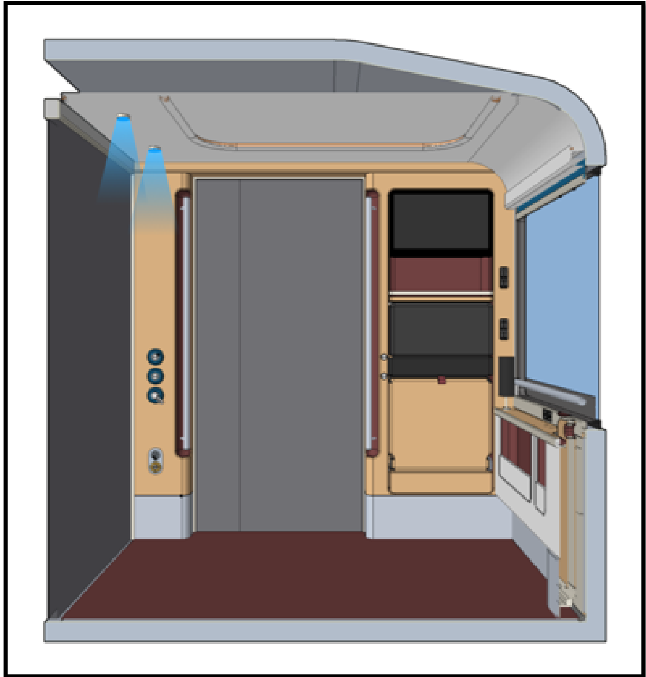
Figure 11-112: Accessible Double Spot Light Locations
