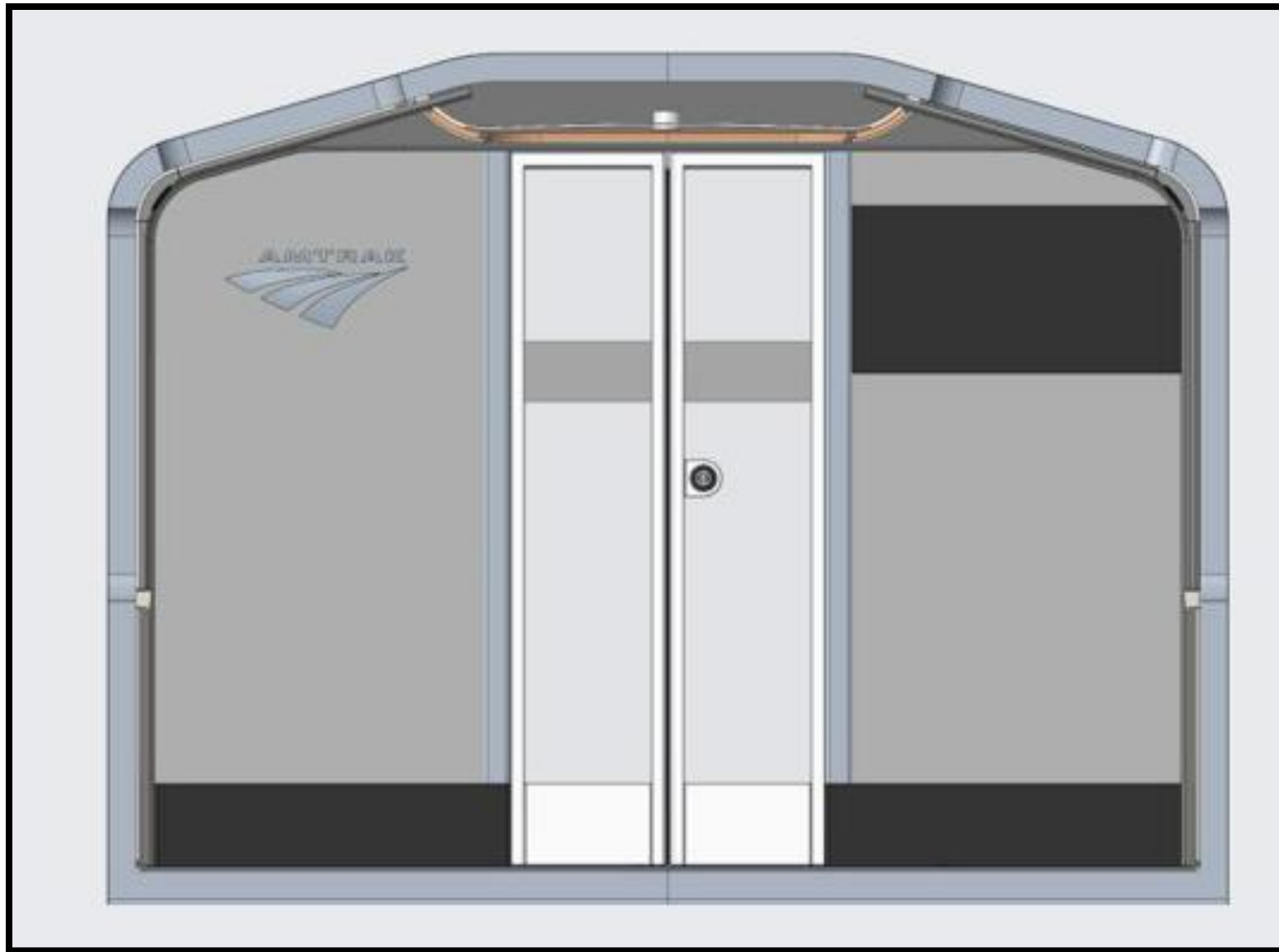
Figure 11-49: Bulkhead Walls with Doors
