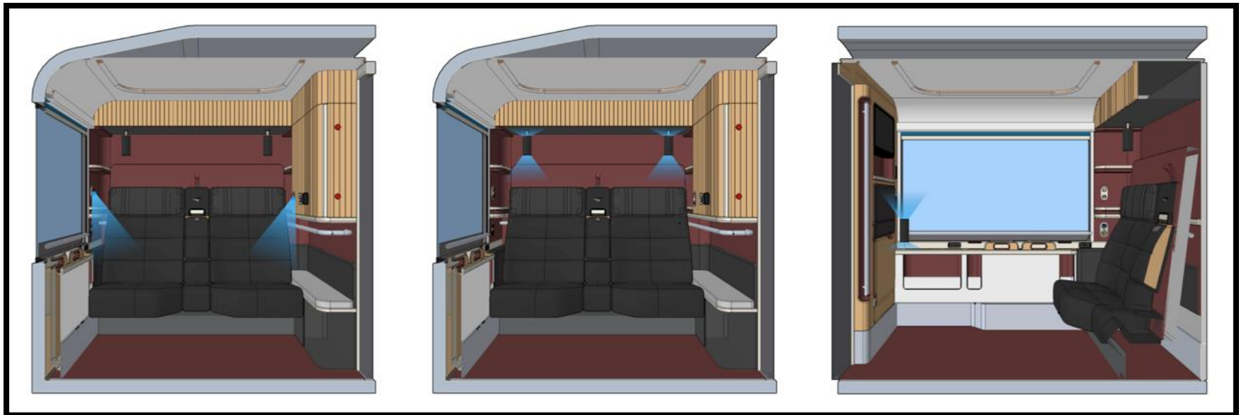
Figure 11-114: Accessible Double Reading Light Locations
