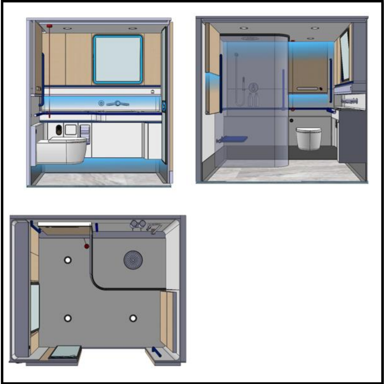
Figure 11-107: Accessible Sleeper Cabin Restroom Lighting
