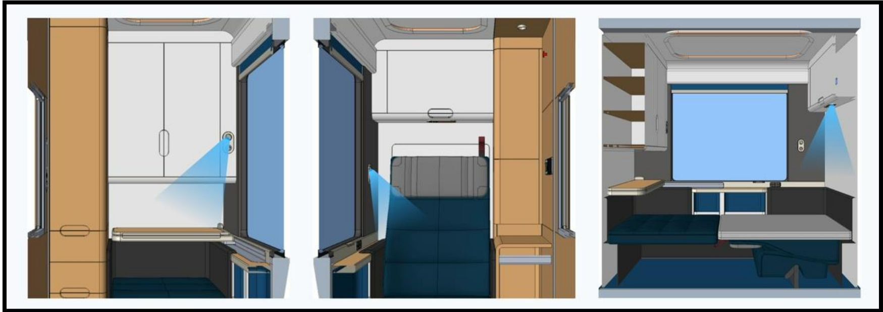
Figure 11-132: Crew Sleeper Reading Light Locations
