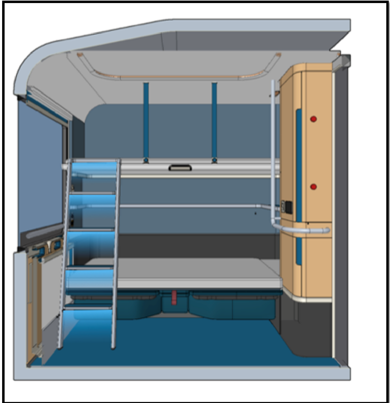
Figure 11-106: Accessible Twin Ladder Light Locations
